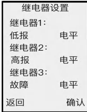
Figure 3. 8 -relay setting interface
