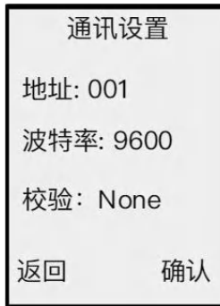
Figure 3.11 Communication settings interface
